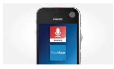
The software development kit (SDK) allows you to customize your existing app to use the different microphones, speakers, slide switch, function key, microphone sensitivity and LED.
