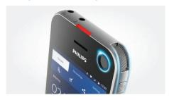
Three professional microphones deliver ultimate sound quality in any recording situation. The 360° microphone is ideal for recording dictations and meetings. The direction microphone is best suited for noisy environments. For VoIP telephony the SpeechAir uses a dedicated microphone.
